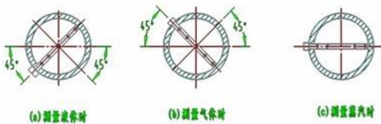
Figure 2. Installation directions of different media
