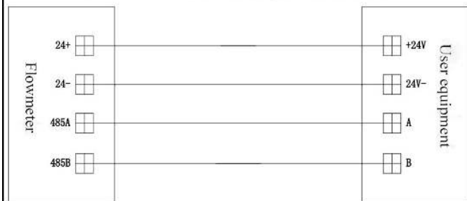
Four-wire 485 communication wiring universal(old models)
