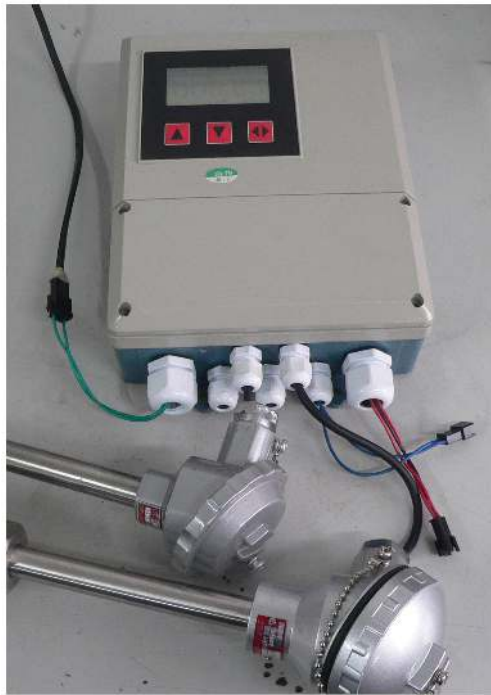
Figure 4.3 The whole picture of electromagnetic flowmeter heat meter
