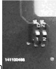
Figure 2.1 Communication resistance switch
