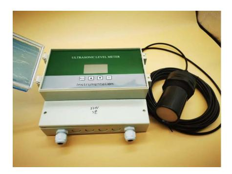
Split type ultrasonic level meter is an intelligent non-contact level measurement instrument.
